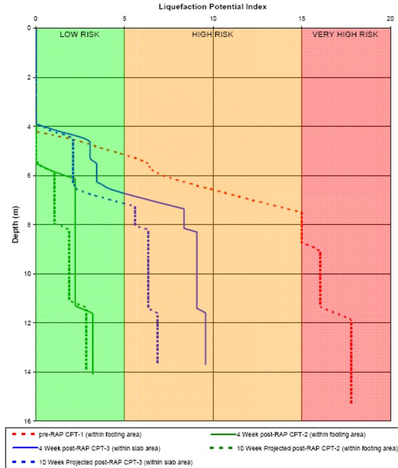
**Figure 4. Pre- and Post-RAP Liquefaction Potential Index**
