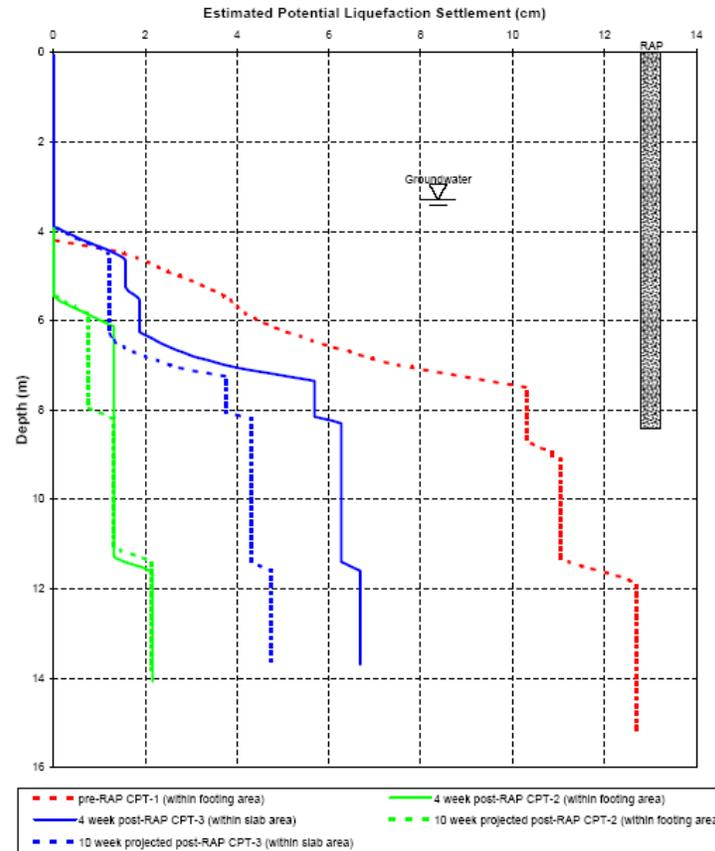
**Figure 5. Pre- and Post-RAP Liquefaction Settlement of Surrounding Soil**
